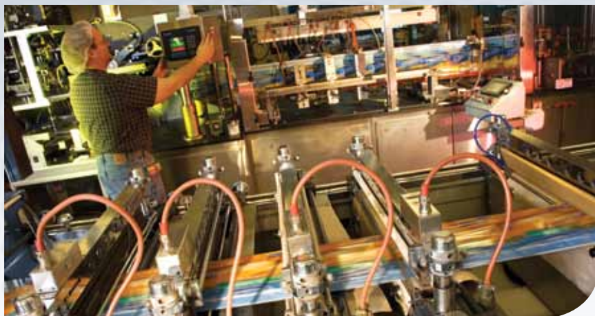
The Mamata Vega 610 (foreground) converts press to close pouches at competitive speeds.
